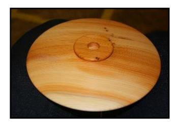
The ring was removed and the top was mounted by the spigot in the chuck with a piece of paper towel between the wood and chuck for protection. A bowl gouge was used to hollow out the dish shape. Again this was shear scraped and sanded to a finish as before.
